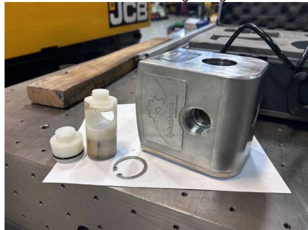
4. Clear Bore and Spool Using Soap/Water
